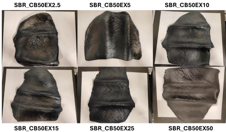
Fot. 2 Illustration of uncured samples with various filler loading ratio. Good processability even at textile loading of 50phr (EX50)
